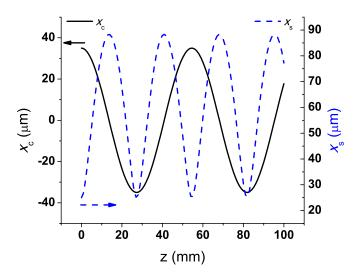
FIG. 1. (Color online) Laser centroid offset  $x_c$  (solid line) and spot size (dashed line) as a function of propagation distance z in a channel of matched spot size  $r_m=47 \ \mu m$  for an input centroid offset of  $x_{ci}=35 \ \mu m$ , input injection angle  $\theta_i=0$ , and initial spot size  $r_i=25 \ \mu m$ .
