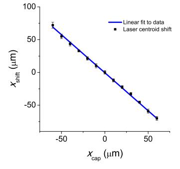
FIG. 7. (Color online) Measured centroid shift (squares), as a function of input laser centroid offset for a capillary of diameter 300  $\mu$ m and length 15 mm and delay 225 ns. The linear fit (solid line) is equivalent to fitting a parabolic shape to the channel.
