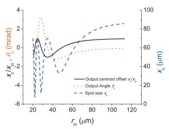
FIG. 2. (Color) Laser beam parameters at the output of a plasma channel of length 15 mm as a function of matched spot size. Normalized laser centroid offset  $x_c/x_{ci}$  (solid line), angle (dotted line), and spot size (dashed line) are shown for an input centroid offset of  $x_{ci}=10 \ \mu$ m, input injection angle  $\theta_i=0$ , and  $r_i=80 \ \mu$ m.
