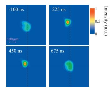
FIG. 5. (Color) Typical laser modes at the output of the capillary for the parameters of Fig. 6. The delay between the discharge and laser pulse is shown at the top left of each image. The dashed line is at a constant location in the image. The centroid shift and spot size reduction is clear for delays during the discharge current.
